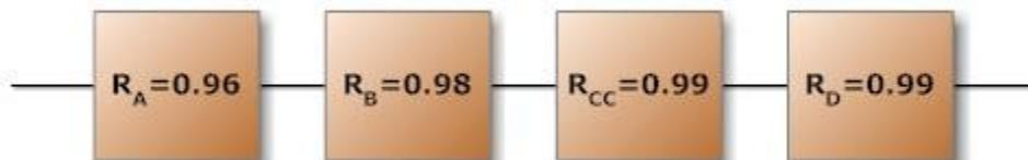
Using the calculation above for the two Cs combined; we can now compute the reliability of the entire system using the equivalent parallel system shown above as follows:
