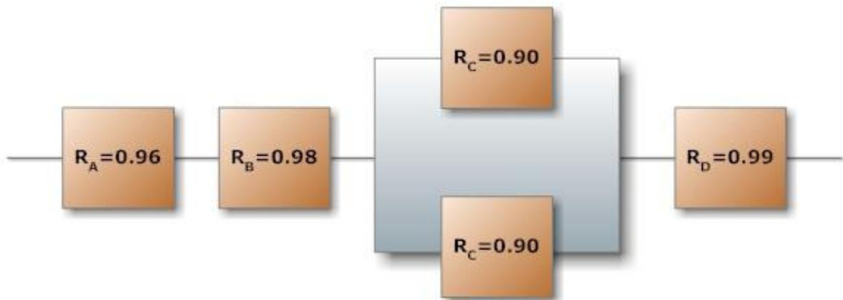
First we must compute the reliability of the parallel subsystem C:
